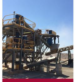
**Crushed Ore Sampling System**
